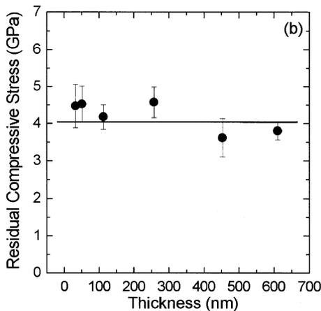
Fig. 1. Dependence of the residual compressive stress on film thickness: (a) a-C:H film deposited by r.f.-PACVD; and (b) ta-C film deposited by FVA.
