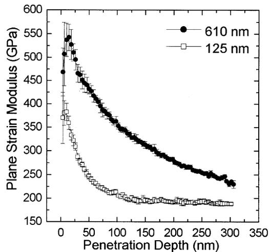
Fig. 7. Plane strain modulus of ta-C films of thickness 610 and 125 nm, respectively, measured by continuous stiffness measurement (CSM) mode of nanoindentation.
