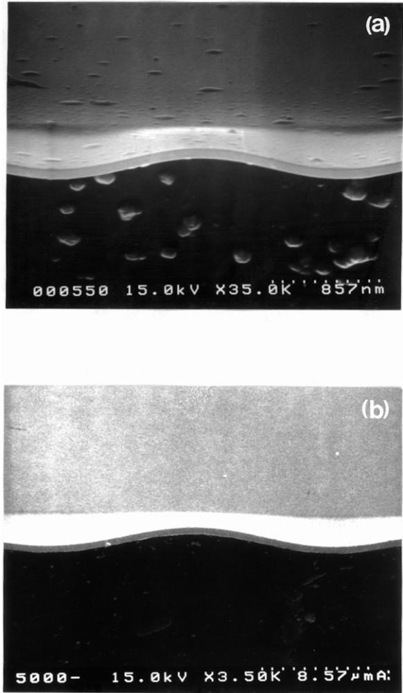
Fig. 2. Typical microstructure of the free overhang of the film deposited by r.f.-PACVD: (a) the film thickness is 55 nm and the etching depth = 2 μm; and (b) the film thickness is 546 nm and the etching depth = 11 μm.
