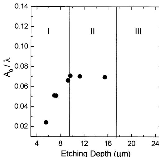
Fig. 3. Typical values of  $A_0/\lambda$  for various etching depths. The data were obtained with a film of thickness equal to 546 nm deposited by r.f.-PACVD.
