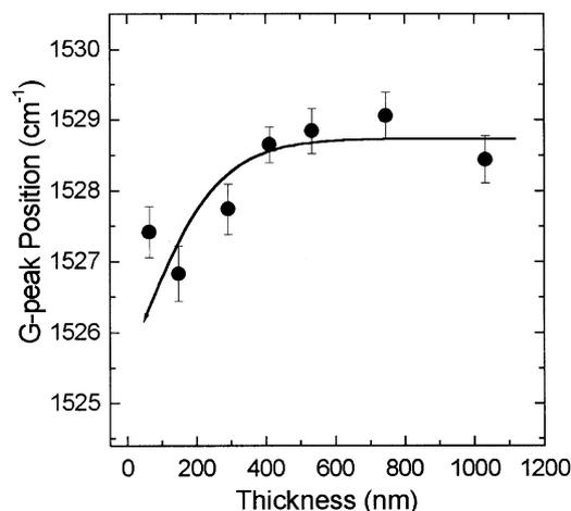
Fig. 5. Dependence of the G-peak position of Raman spectroscopy on the a-C:H film thickness.
