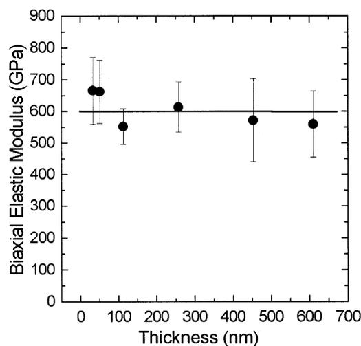
Fig. 6. Calculated biaxial elastic moduli of ta-C films for various film thicknesses.
