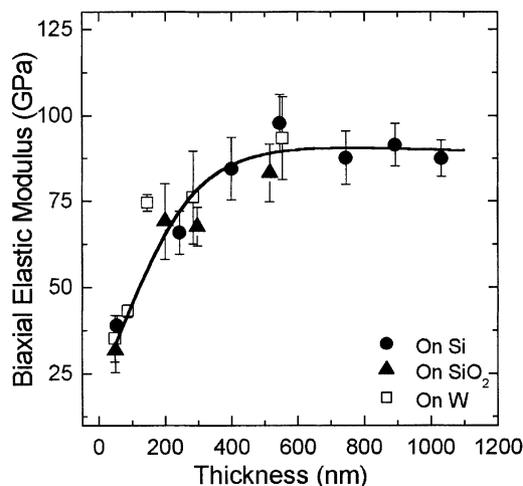
Fig. 4. Calculated biaxial elastic moduli of a-C:H films for various film thicknesses and substrate materials.
